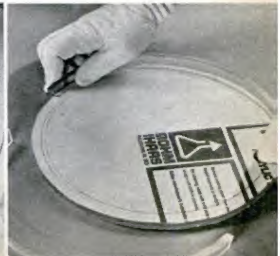
SUPPORT COLLAR , on which top rests at center, has two shaped plastic strips glued together
